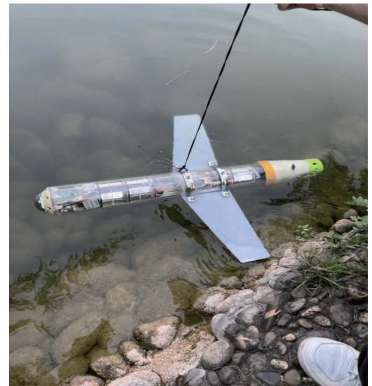
Figure 4: Underwater water quality intelligent monitoring system hull launching test
