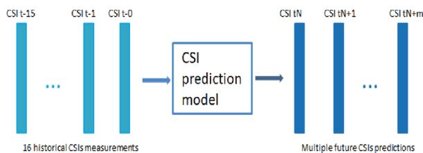
Figure 1 AI based CSI prediction block diagram
